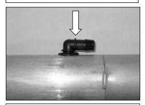
n. Insert the 1" grommet into the pipe. Insert the 90 degree plastic connector into the grommet. Be careful not to push the grommet through the pipe.
