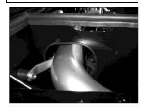
o. Insert the pipe as shown. Line up the support bracket to the rubber mount and secure. See diagram on next page.
