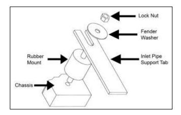
Proper installation of rubber mount assembly.
