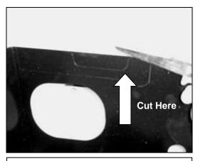
f. Trucks equipped with the optional under hood light on the *passenger side*, cut the corners on the small section of the top notch in the heat shield using a hacksaw or other suitable tool. Bend the tab back and forth until it breaks free. Clean up any sharp edges with a file. Vehicles not equipped with the under hood light, proceed to next step.
