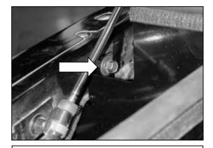
k. The rear mounting tab on the heat shield will line up with one of the lower air box mounting holes. Install one of the original bolts. Adjust the heat shield for best fitment then tighten the three mounting bolts.
