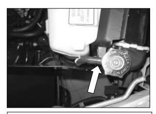
i. Disconnect the overflow tube to gain access to the upper radiator fan shroud bolt. Install the heat shield from inside the fender well. Place the front heat shield tab between the fan shroud and radiator end tank. Replace the factory bolt and overflow bottle.
