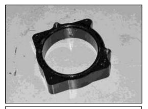
c. Install the supplied o-ring into the groove in the front of the throttle body spacer. Make sure the o-ring is properly seated in the groove around the entire circumference. Use a small amount of grease to trap the o-ring in place.
