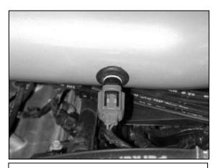
p. Reconnect the wire harness to the IAT sensor. Do not push the grommet through the pipe.
