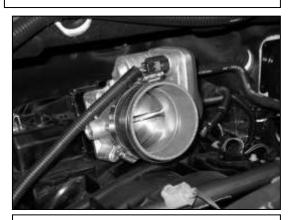
m. Loosely install the coupler and hose clamps onto the throttle body. Secure with provided hose clamps.
