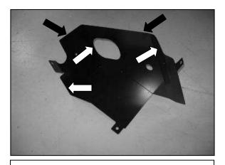
g. Install the rubber edge trim (PN: 8-4022) on the edges indicated with the white arrows. Install the sponge rubber gasket (PN: 8-3034) along the top of the heat shield indicated with black arrows.
