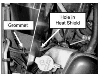
b. Pass both connectors through the supplied large grommet and then through the hole in the heat shield. Reconnect wire connectors and washer fluid hose to the washer fluid reservoir.
