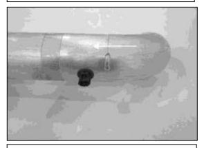
I. Install the supplied IAT grommet into the inlet pipe. Insert the factory IAT sensor into the grommet. Use care to avoid pushing the grommet into the pipe.
