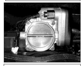
j. Remove the four bolts securing the throttle body. Unplug the electrical connector and remove the throttle body from the intake manifold.
