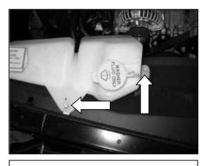
h. Loosen and remove the overflow reservoir mounting bolts.
