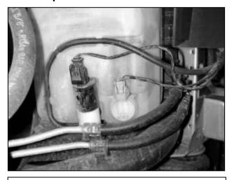
a. Unplug the wire connectors going to the windshield washer fluid pump and level indicator. Unplug the washer fluid hose. Block the nipple on the pump to prevent the washer fluid from draining.
