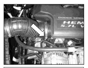
b. Loosen the hose clamp at the intake air resonator. Remove the rubber air hose and the air box lid.
