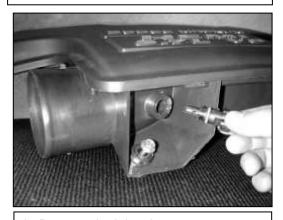
h. Remove the inlet air temperature (IAT) sensor from the intake resonator by gently twisting counter-clockwise. Remove the o-ring from the IAT sensor. Keep the o-ring for use if the vehicle ever needs to be returned to stock.
