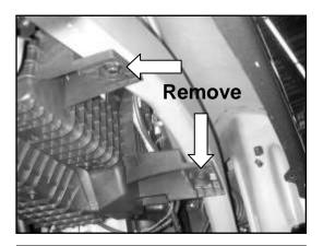
d. Remove the two bolts securing the bottom half of the air box.
