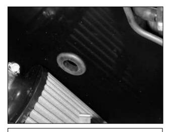
c. Install the rubber grommet in to the hole in the heat shield. Make sure the groove in the grommet is properly seated in the heat shield.
