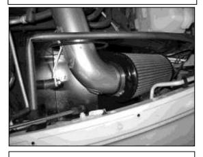
s. Install the air filter from inside the fender well. Slide the air filter on to the pipe until it stops. Secure with the supplied hose clamp. Make sure the windshield washer wires and hose do not come into contact with the air filter.
