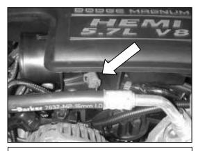
f. Unplug the inlet air temperature (IAT) sensor located on the front side of the intake air resonator.
