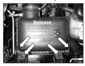
a. Release the four spring clips that hold down the top of the air box.
