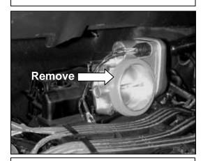
i. Remove the orange rubber gasket from the throttle body.
