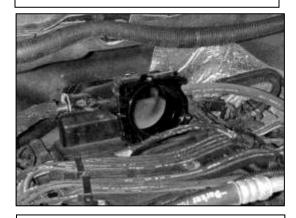
d. Install the throttle body spacer, aligning the pins on the intake manifold with the holes in the back of the throttle body spacer. The o-ring groove on the spacer should be facing forward.
