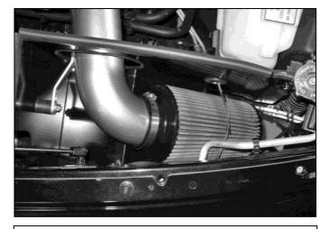
d. Install the air filter. Adjust the windshield washer hose and wires so they do not rub against the air filter.
