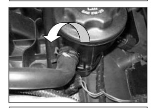
r. To increase the clearance of the breather hose and the inlet pipe, rotate the breather line at the PCV outlet counter clockwise. Release the spring clamp to rotate.
