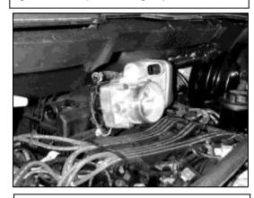
e. Install the throttle body using the supplied M6 bolts and washers. Align the dowel pins on the throttle body spacer with the holes in the throttle body. Before installing the throttle body spacer, make sure the o-ring is seated. Reconnect the electrical connector.
