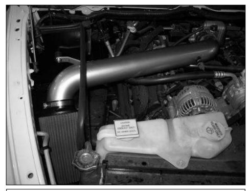
AEM® intake system installed
