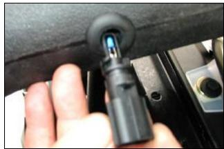
**9.** <u>2003-2005 Models Only:</u> Install rubber grommet w/thru hole and insert the factory air temperature sensor into the grommet.
