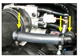
**15.** <u>2002 & 2003 Models Only:</u> Use the 90° plastic elbow provided, connect the factory breather hose with the 4 ½" hose to the Airaid tube & secure using the three #16 black Speed clamps.
