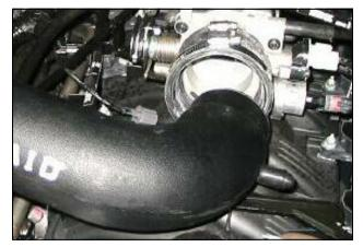
**13.** Position Airaid tube into place by connecting hump hose to Airaid Cool Air Dam and connect the other end of the tube to the factory throttle body coupler. Utilize the #60 hose clamps on the hump hose and #56 hose clamp on the factory coupler.
