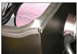
**18.** <u>2004-05 Models Only:</u> Connect the factory breather hose to the Airaid Cool Air Dam & secure using the #24 Speed clamp provided.
