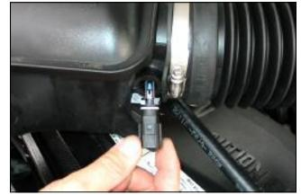
**6.** <u>2003-05 Models Only:</u> Disconnect air temperature sensor wire on back of factory throttle body air chamber and remove sensor. Retain sensor for later use with the Airaid Intake System.
