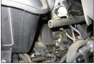
**5.** <u>2002 & 2003 Models Only:</u> Disconnect the crankcase vent hose on the back of the factory throttle body air chamber.
