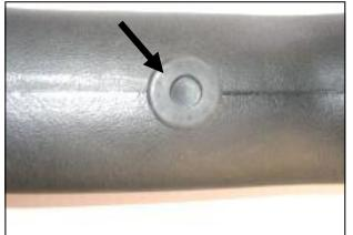
**8. 2002 Models Only:** Install rubber grommet plug into the hole on the side of the Airaid tube.
