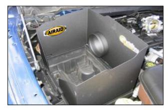
**10.** Position the Airaid Cool Air Dam in place of the original air box lid. Snap in place.
