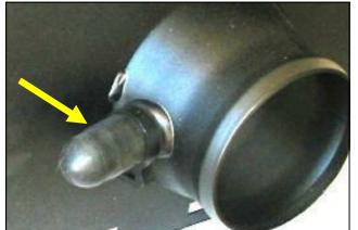
17. <u>2002 & 2003 Models Only:</u> Slip the black rubber cap over the nipple on the Cool Air Dam and secure using the #19 Speed clamp provided.
