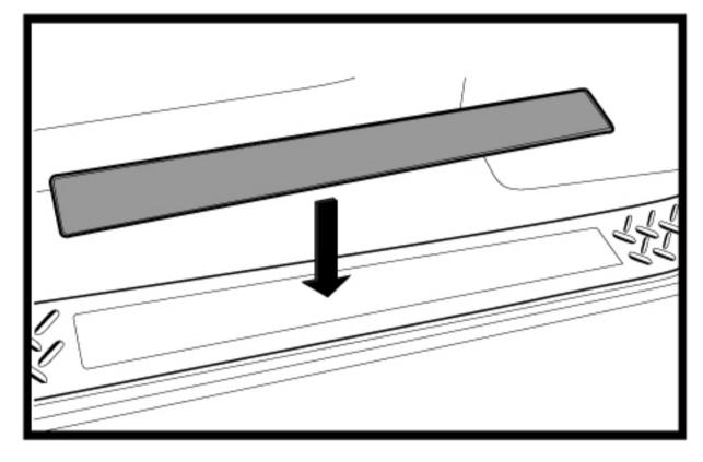
Accurately measure the sill plate position prior application. Repositioning of the double-sided tape can deteriorate their adhesive property.
