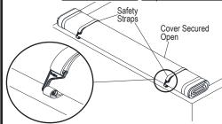
Secure cover open by hooking safety straps to front loops.
