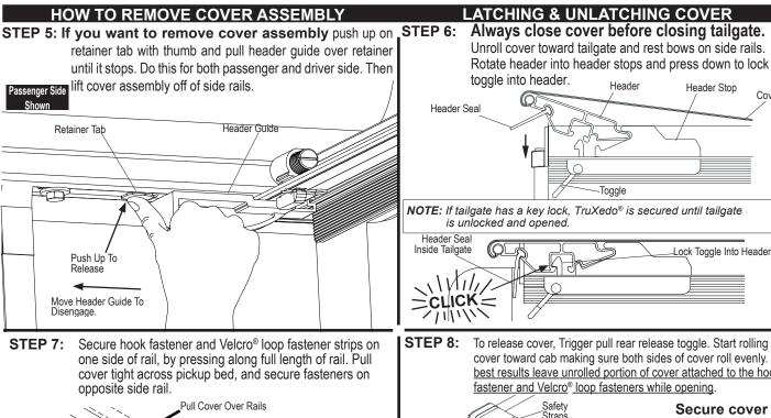
Press Edges Hook and Loop Fastener NOTE: Secure hook fastener and Velcro® loop fastener along entire length of both side rails before driving vehicle. This will prevent wind lifting Toggle the cover and causing damage.
