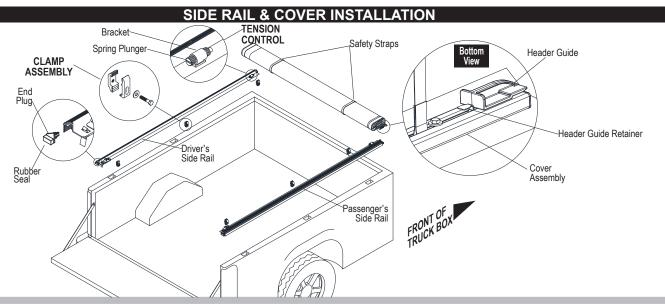
STEP 1: Attach the TruXedo rails to the truck's vertical inside flange as shown in Detail A. To get the correct TruXedo rail alignment from front to back, See Detail-B. Compress the rear D-seal against the closed tailgate and hold. Attach clamps starting at the tailgate. Evenly space 3 clamps along each TruXedo rail, leaving approximately 8" on each end.
