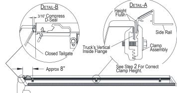
For optimum latching performance and cover fit, side rails must be level. To adjust rails, loosen screws and reposition male clamps higher or lower. Tighten all clamps.
