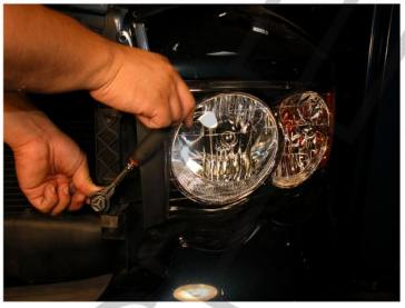
3. Then remove the two 10 mm bolts from the headlight
