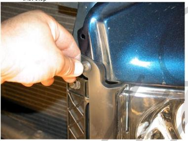
7. Install the clip to fasten the headlight
