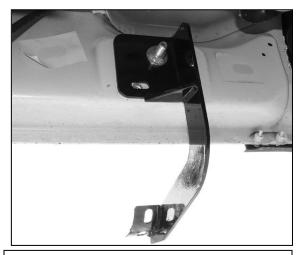
(Fig 3A) Driver/Left front Mounting Bracket
