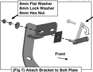
Remove Hex Bolt, rotate Bolt/Nut Plate to line up threaded nut with body panel and Mounting Bracket (see arrow)
