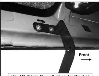
(Fig 15) Attach Driver/Left center Bracket
