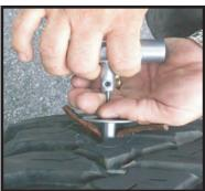
(6) Cut off ends of rubber plug at tread. Slowly inflate tire and checking for leaks.
