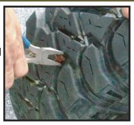
(2) Remove object from tire. For on road repairs hole must be located 1" inbound from either edge of tire tread. DO NOT REPAIR if hole is located near or on the sidewall of tire.
