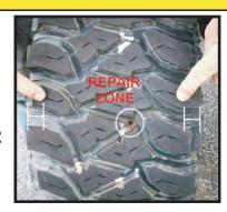
(3) Insert T-handle punch into hole. Work punch in and out several times to clear hole for plug.
