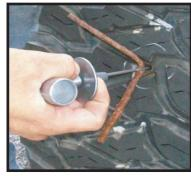
(5) Press down on plunger extractor and pull up on T-handle to insert rubber plug into tire.
