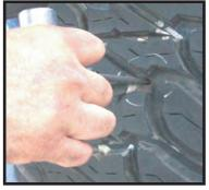
(4) Insert rubber plug into eye of T-handle plunger. Place plunger eye into hole and insert to base of plunger extractor.
