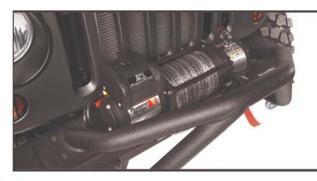
Rugged Ridge All Terrain Bumper base with Double-X Striker and a 12,500LB Winch
