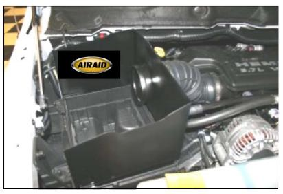
**4.** Install the **Quick Fit Panel** (#2) by slipping it into the factory intake tube, and then sliding it over the tabs on the factory airbox base. Adjust it for fit on top of the airbox base, and re-latch the 4 clips to hold the **Quick Fit Panel** securely in place. Apply the Airaid Foil Decal onto the Panel as shown.
