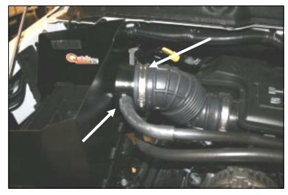
5. Slide the factory intake tube all the way onto the Quick Fit Panel tube and tighten the hose clamp. Slip the #24 speed clamp(#4) over the factory breather hose and re-connect the factory breather hose to the nipple on the Quick Fit Panel. Squeeze the speed clamp to secure the breather hose.
