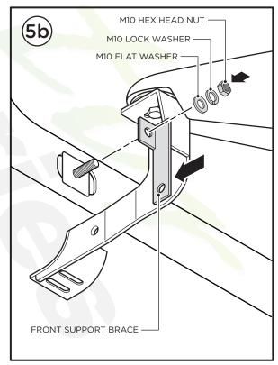
**6.** Fasten the Front Support Brace to the Front Bracket using one (1) M10 Lock Washer, two (2) M10 Flat Washers, one (1) M10 Hex Head Nut and one (1) M10 x 30MM Hex Head Bolt.
