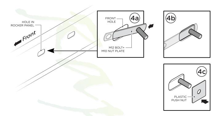
**5.** Locate hole in the rocker panel and insert one (1) Bolt Plate with M12 Stud into the hole (5a) and (5b). Slide Plastic Push Nut over the Stud (5c). Repeat for Rear Bracket.
