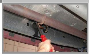
Unbolt the downpipes/cats from the exhaust manifolds. Using a pry bar, slide the whole exhaust system back on the metal rod hangers. Move it back far enough that the exhaust manifolds can be removed. It just takes a few inches and its out of the way. NOTE!!! Be sure to use WD-40 on the hangers to allow the exhaust system to slide back easier.
