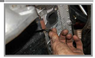
To aid in the installation, the 2 rear bottom bolts need to be threaded halfway into the head because the tight fit of the tube will not allow them to be installed after the header is fully on. This needs to be done on both sides of the engine. Use the provided header bolts. You can install the gaskets on the head and hold them down with the pre-installed bolts.
