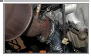
Work the exhaust system back up to the headers. Connect the stock exhaust flanges to the BBK Headers using the provided hardware. Tighten the collector studs on both sides, drawing the downpipes tight as you do, and reconnect the oxygen sensor plugs.
