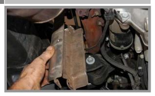
Remove the four nuts that hold the heat shields to the exhaust manifolds and remove them.
