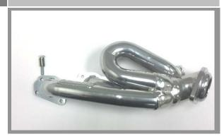
Lower the vehicle down and re-install the dip stick tube. NOTE!!! On 2009-2014 use the supplied spacer and longer header bolt, reinstall the dip stick tube on the top front header bolt hole as shown above.
