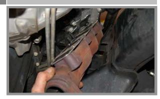
Unbolt both exhaust manifolds and remove from the vehicle. Also remove the stock gaskets.
