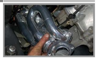
On the driver side, the steering shaft needs to be unbolted and moved to the side and the engine needs to be lifted. Install the supplied gasket and BBK Header into place and tighten in an X-pattern. <u>NOTE!!!</u> On 2009-2014 Models Leave the front top hole with no bolt. The longer header bolt that is supplied will be used when re-installing the dip stick tube.
