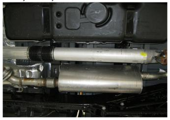
**Step 3.** You are now ready to install your new MAGNAFLOW system. Loosely attach the the Muffler Assembly to the OEM pipe outlet using the supplied 3.00" clamp. Be sure to line up the large notch in the pipe wiht the alignment peg. Engage the welded hanger to the OEM rubber insulator. Leave all clamps and hardware loose for final adjustment of the complete system.
