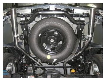
**Step 6.** Loosely attach the polished tips using the supplied 2.50" clamps to the desired position.
