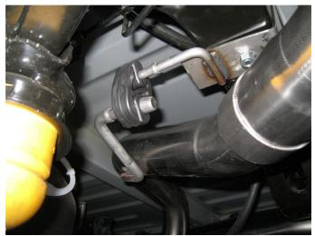
**Step 5.** Install both Tail Pipe Assemblies in a similar fashion. Use the supplied rubber Insulator to locate the drivers side welded hanger.
