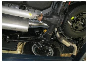
**Step 1.** Begin removing the OEM exhaust by unbolting the clamp attaching the tail pipe assembly. Disengage the welded hangers from the OEM rubber Insulators using a pry bar or similar tool. Remove the assembly.
