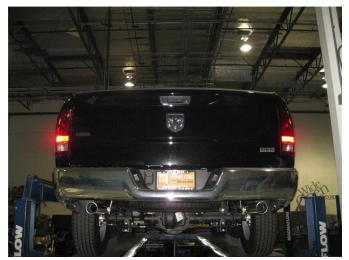
**Step 7.** Once a final position has been chosen for the new system, evenly tighten all fasteners from front to rear using the torque specifications on page one of this document. Inspect all fasteners after 25-50 miles of operation and retighten if necessary.
