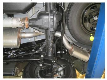
**Step 2.** Unbolt the clamp just behind the muffler. Do not damage or discard the OEM fasteners or rubber insulators, as they will be reused to mount the new system. Disengage all hangers and remove the OEM system from the vehicle.
