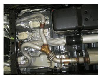
**Step 1.** To remove the OEM exhaust system, you will first need to unbolt the muffler assembly from the Y-Pipe assembly.
