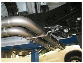
**Step 5.** Next, install the Tail Pipe Assembly by slipping the inlets over the Muffler Assembly outlet pipes. Loosely secure with the supplied clamps. Locate the supplied rubber isolator to the previously mounted hanger and the welded hanger on the assembly.
