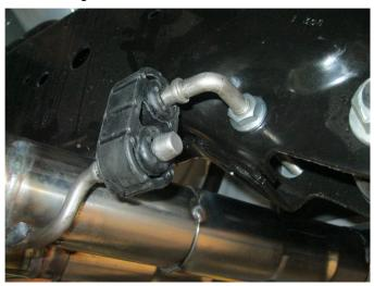
**Step 4.** To support the Tail Pipe Assembly you will need to locate the supplied threaded hanger through two exsisting holes in the vehicles sub frame. Secure with the supplied hardware as shown.
