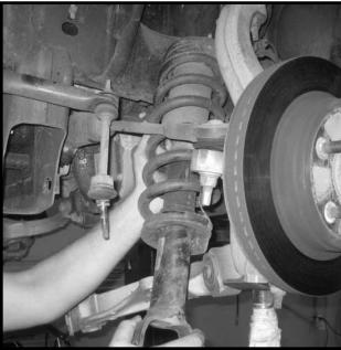
8. Install the new front spacers on the coil overs using the OE hardware. Make sure to use loctite and torque to **32 ft lbs.**
