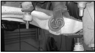
5. Working on the driver side, place a reference mark on the cam washer and cam stops that attach the lower control arm to the front and rear lower control arm mounts. Repeat procedure on the passenger side.
