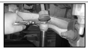
4. Working on the driver side, remove the hardware that attaches the coil over to the lower control arm. Save the hardware. Repeat procedure on the passenger side.
