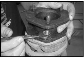
9. Locate (6) 3/8 nylon nuts and (6) 5/16" USS flat washers from hardware bag D2P-NB. Working on the driver side, install the newly modified coil over into the upper location and secure using the new hardware. Make sure to use loctite and torque to 32 ft lbs. Repeat procedure on the passenger side.
