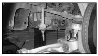
7. Working on the driver side, remove the (3) nuts that attach the coil over into the upper location. Save the hardware. Remove and set the coil over aside. Repeat procedure on the passenger side.
