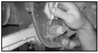
6. Working on the driver side, remove the hardware that attaches the lower control arm to the front and rear lower control arm mounts. Save the hardware. Repeat procedure on the passenger side. **Special note: Let the lower control arms hang and rest on the hydraulic floor jacks.**
