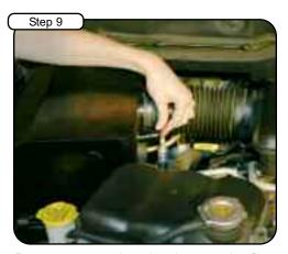
Re-connect your breather hose to the filter nipple. If your vehicle is not equipped with a breather hose, cap off the nipple with with the supplied vacuum cap.
