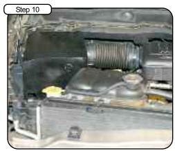
Place enclosed CARB EO sticker on a clean/smooth surface on or near the intake system. EO identification label is required to pass the smog inspection.
