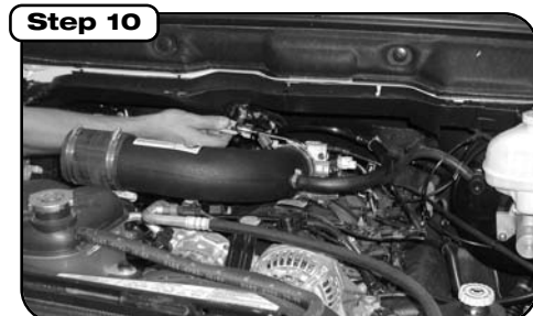
Place Intake tube "L" Bend in place. Tighten hose clamp and connect temperature sensor if applicable.
