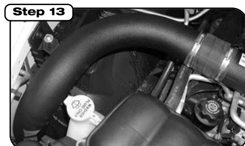
Lower the "S" Tube into place with the attached tabs towards the front. Join the tubes with the 3-1/2" x 4" straight coupler. The remaining M8 Nuts, lock washers and flat washers can now be installed
