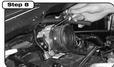
Remove stock resonator boot.
