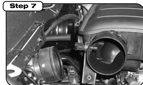
To remove resonator lift up to free the front grommet and pull out.
