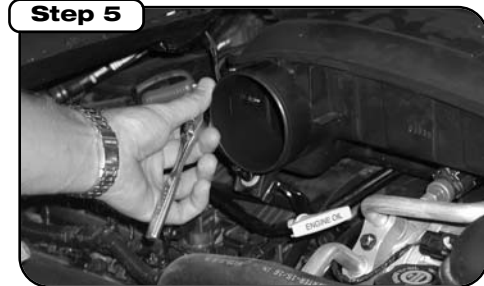
Remove the two resonator hold down bolts.
