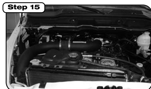
Place enclosed CARB EO sticker on a smooth/clean surface on or near the intake system. Eo identification label is required in passing Smog Check inspection. Make sure all hoses and clamps are tight and that all electrical components are secure. Re-check and after a few hours of operation.
