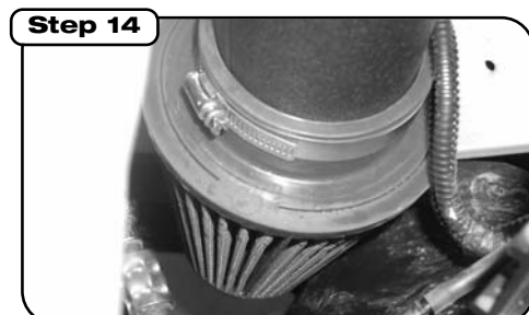
Install the filter from below the vehicle and tighten the clamp from above. Make sure the clamp is at the upper edge of the filter so that it doesn't slip off.
