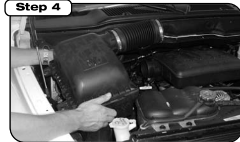
Pull off boot from resonator box and remove complete filter box assembly.
