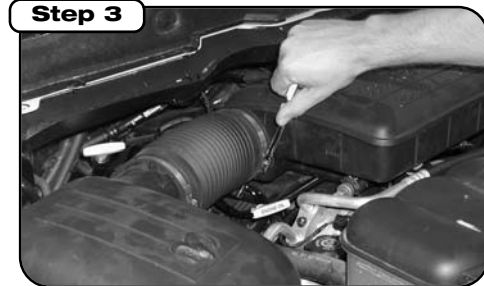
Loosen clamp at resonator box.
