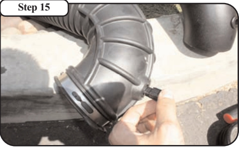
zRemove the temperature sensor from the stock intake tube. Use a rag to help pull the sensor straight out. The sensor is plasic so take your time and be careful when removing.
