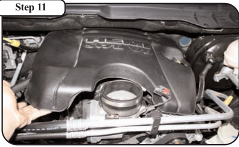
Remove the engine cover by pulling up on one side at a time to pop it loose. Install the 15deg elbow coupling on the throttle body and leave the clamps loose.
