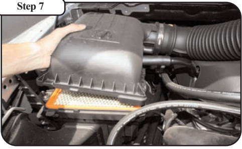
Lift off the stock air box cover and tube.
