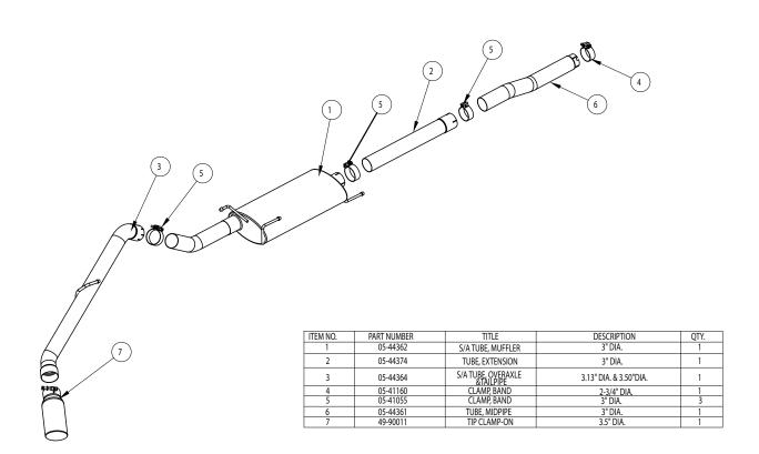
**Step 1:** (**Read Instructions prior to installation**) Remove your stock exhaust from the rear of your truck working your way forward. It may be necessary to cut the pipes if the slip joints are stuck. Do not cut the pipe after the cat. You will be using this slip connection. Take caution not to damage the factory isolation mounts, as they will be reused. It is recommended to not fully tighten the clamps until the entire system is installed.
