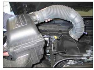
5. Disconnect the factory intake hose from the throttle body, then lift up the air box assembly and remove from the vehicle.
