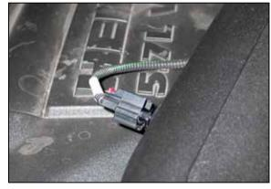
27. Connect the provided inlet temperature sensor extension into the factory wiring harness and then connect the other end to the inlet temperature
