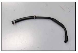
9. Install the provided crank case vent hose onto the cut end of the factory crank case vent tube with the provided hose clamps as shown.
