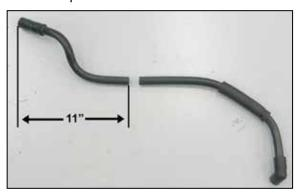
8. Measure 11" from the air filter end of the crank case vent tube and then trim the crank case vent tube as shown.
