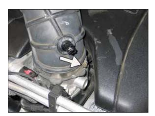
3. Loosen the hose clamp that secures the intake tube to the throttle body.
