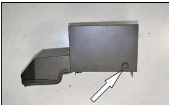
11. Install the factory rubber mounting grommet into the K&N® heat shield as shown.
