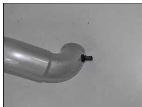
20. Install the inlet air temperature sensor into the grommet installed into the K&N® intake tube. NOTE: Remove the factory sealing O-ring from the sensor before installation.
