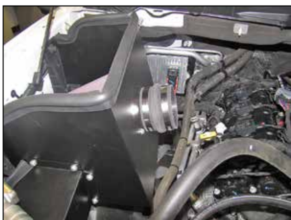
16. Install the provided silicone hose (08699) onto the filter adapter and secure with the provided hose clamp.
