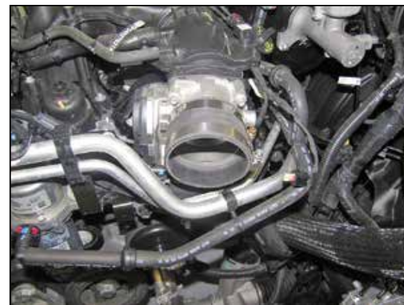
17. Install the provided silicone hose (08690) onto the throttle body and secure with the provided hose clamp.
