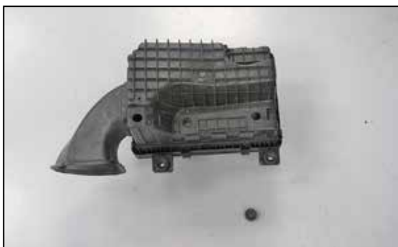
10. Remove one of the rubber mounting grommets from the factory air box.
