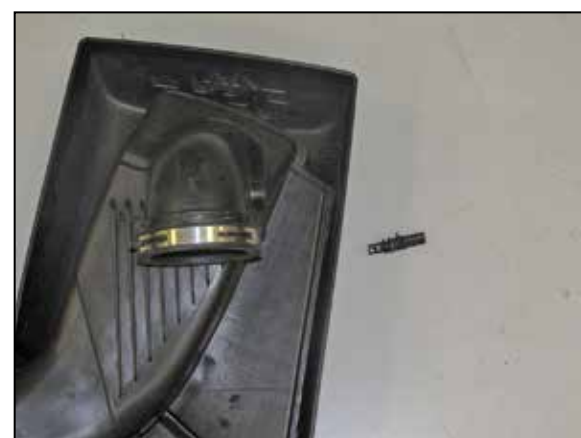
19. Remove the inlet air temperature sensor from the factory intake plenum.
