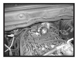
Step 10 Install the 3.5" coupler (5.7L engine) on the throttle body. If you have a 4.7L engine, install the 3.25"- 3.5" reducing coupler then install the 3.5" coupler. Tighten the clamp on the throttle side and make sure the intake side clamp is installed but left loose.
