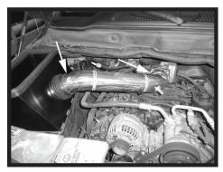
Step 12 Install the Spectre Performance intake tube into the coupler on the heat shield and then into the throttle body coupler. Once in position fully tighten the clamps.
