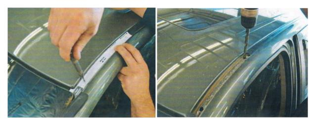
7. Take the supplied 5/16"x 1" bolt, washer, and 3/8" nut and screw them into the nut insert.
