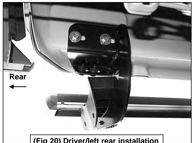
(Fig 20) Driver/left rear installation
