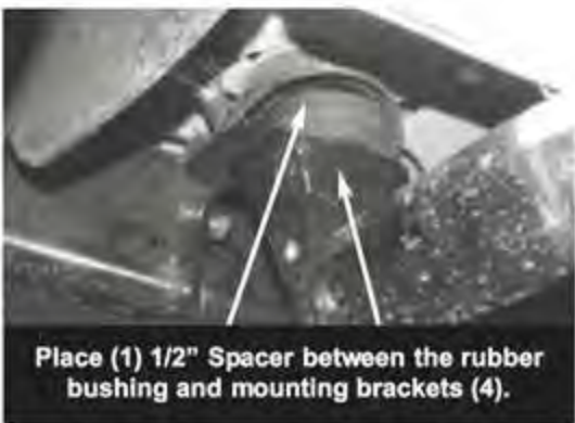
Figure 4 - 1/2" x 1.88 x 3/16" Spacer
