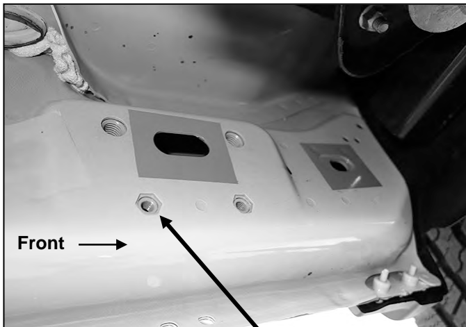
(Fig 8) Driver side front mid 2015-on, an example of models with factory installed threaded inserts
