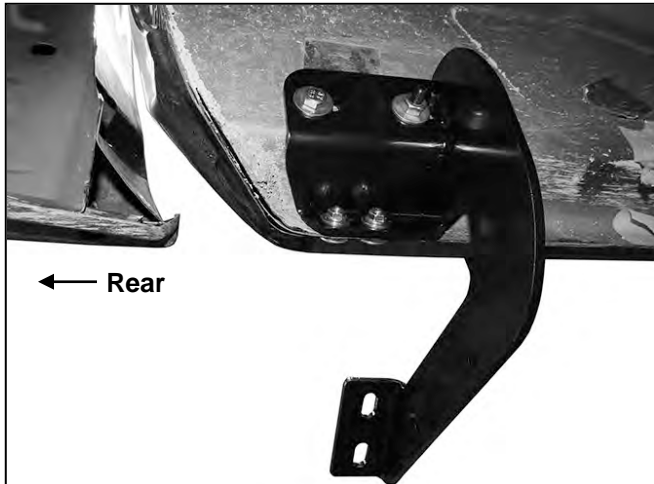
(Fig 16) Driver/Left rear Mounting Bracket assembly
