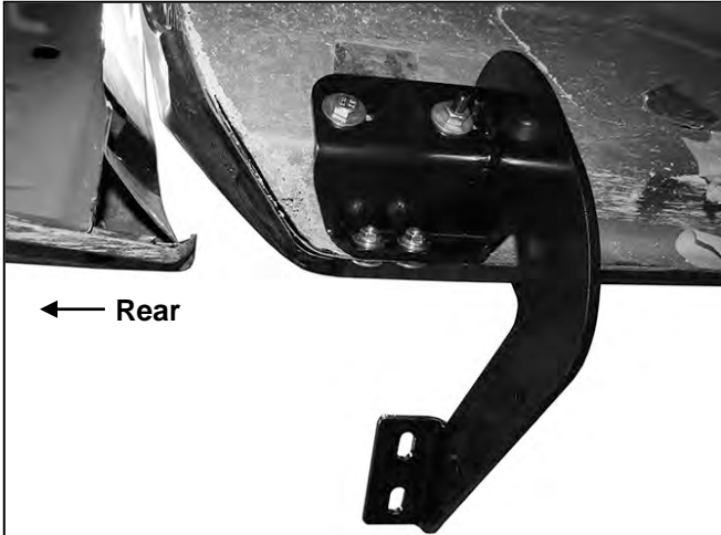
(Fig 16) Driver/Left rear Mounting Bracket assembly
