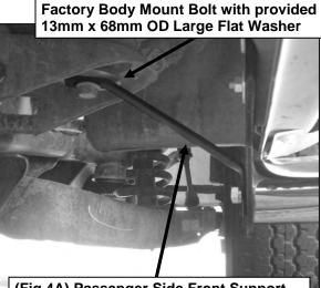
(Fig 4A) Passenger Side Front Support Bracket installation pictured
