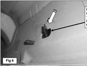
Remove tape covering mounting location. Insert 10mm Bolt Plate W/Bend into the oval hole and out the round hole
