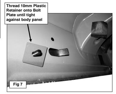
10mm Bolt Plate W/Bend 10mm Lock Washer 10mm Flat Washer 10mm Hex Nut
