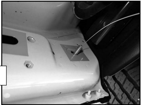
(Fig 2B) Thread 10mm bolt plate onto fish wire. Be careful not to pull other end of fish wire from rocker panel slot
