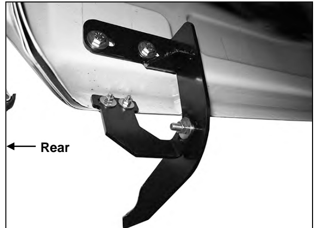
(Fig 18) Driver/Left rear Mounting Bracket assembly
