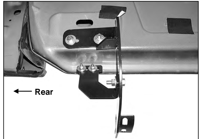
(Fig 18) Driver/Left rear Mounting Bracket assembly
