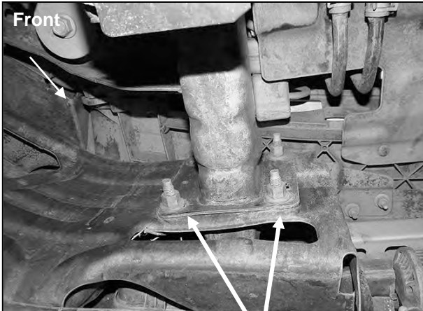
(Fig 5) Remove factory hex nuts from each side
