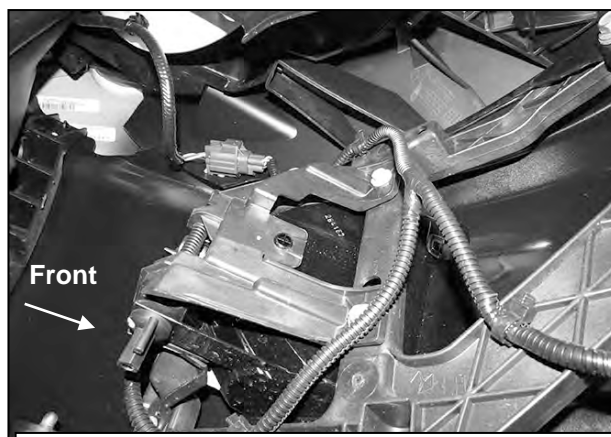
(Fig 2) Unplug fog lights if equipped. Unplug harness to bumper and move harness
