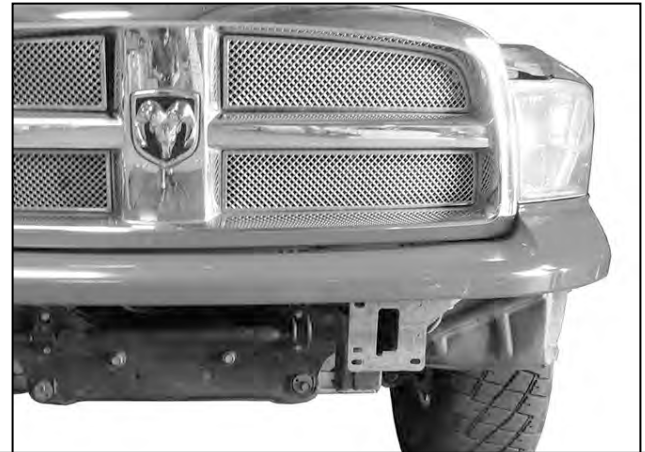
(Fig 6) Remove fascia body panel from top of bumper
