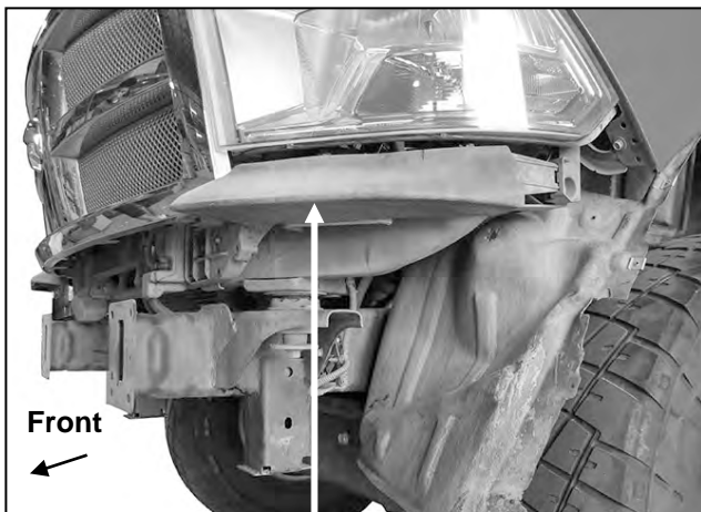
(Fig 7) Remove plastic block from below headlights
