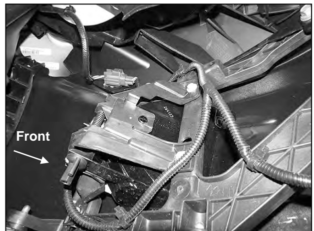
(Fig 2) Unplug lights and sensors if equipped. Unplug harness to bumper and move harness
