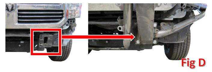
4. Secure the bumper to the frame horns using the supplied 1/2" Bolts (x8), 1/2" Washers (x16), and 1/2" Lock Nuts (x8). Leave these finger tight for now.
