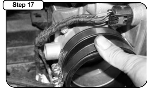
Install supplied coupler and clamps on throttle body, do not tighten
