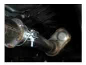
3) Place the provided 3" clamp onto the inlet of muffler **#8530012-395**, then slide onto the factory front pipe and connect the two hangers at the back of the muffler to the rubber mounts on the vehicle. Be sure to line up the notch on the muffler inlet with the tab on the pipe.
