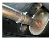
2) Support the muffler with a stand and loosen the clamp on the muffler inlet pipe, then remove the two hangers at the rear of the muffler from the rubber mounts on the vehicle. Slide the muffler to the rear and disconnect from the inlet pipe. Lower and set the muffler aside.
