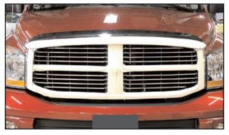
Apply masing tape to the factory grille surround to protect it from scratches while installing the E&G "Q" or "Mesh" grille inserts.
