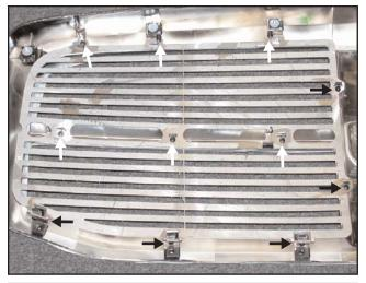
For "Q" Grilles: Drill 1/8" holes and install the supplied 3/4" (white arrows) & 3/8" (black arrows) black truss head screws (where shown).
