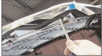
2. Open the hood and remove the twelve 8mm factory fasteners to remove the factory grille surround from the hood (six 8mm hex bolts across the bottom, six 8mm hex nuts across the top). It may be necessary to careful ly cut through the black sealer between the hood and the grille. Place the grille onto a clean, flat work area.
