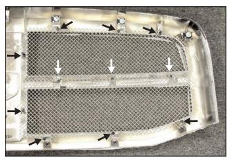
7. For "Mesh" Grilles: Install the mesh grille sections into the factory grille frame by aligning the slots in the mesh grille sections with the existing tabs. Drill 1/8" holes and install the supplied 3/4" (white arrows) & 3/8" (black arrows) black truss head screws (where shown). IMPORTANT: Do not overtighten the screws or you will strip out the plastic grille frame mounting holes! Use the supplied black plastic washers where necessary (may require trim ming).
