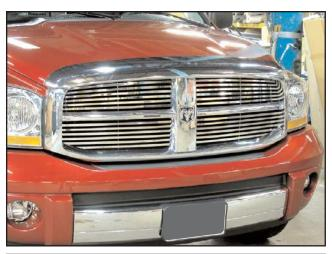
Reinstall the assembled grille frame back onto the hood reusing the factory hardware to finish ("Q" grille shown).
