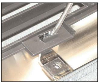
Remove the factory grille inserts from the grille surround using a small flat blade screwdriver to pry the inserts over the tabs on the grille shell.
