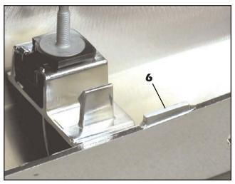
For "Mesh" Grilles: You must first gind the upper tabs (one each side) flush with the factory grille frame in order for the mesh sections to lay flat against the inner edge.
