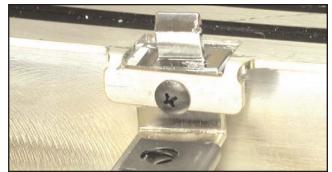
4. For "Q" Grilles: Install the stainless steel E&G grille left and right sections into the factory grille frame by aligning the inner slots in the grille sections with the exist ing tabs. Drill 1/8" holes and install the supplied 3/8" black truss heads screws (where shown in the three lower 90 degree bent tabs first). IMPORTANT: Do not overtighten the screws or you will strip out the plastic grille frame mounting holes!
