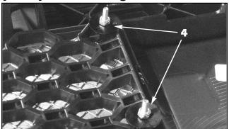
4. Install the stainless steel E&G grille sections into the openings on the factory grilles and tape them into place. Turn the grille over and install a large black plastic washer and a #8-32 ESNA half nut onto each mounting stud and tighten until snug. DO NOT OVERTIGHTEN or you will indent the grilles at the stud locations (mesh grille shown, "Q" grille same).
