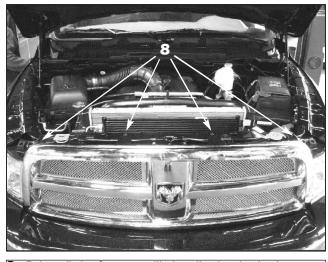
8. Reinstall the factory grille by clipping in the lower edge and reinstalling the four (4) 10mm hex head bolts.
