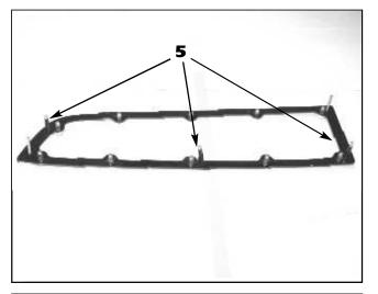
Install the #8 x 1-1/4" black cap plugs once the closed ends have been cut off onto the upper upper grille surround as shown. Install the black cap plugs to the bottom studs on the lower upper grille sur rounds (not shown).
