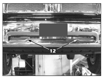
12. Align the mesh sections and the lower surround into the opening in the front bumper. Make sure the studs pass through the holes drilled in the previous step (mesh grille shown, "Q" similar).
