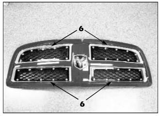
6. For E-Power Grilles: Apply tape around the grille openings and align the mesh and surrounds into place, making sure all six (6) mounting studs per surround pass through the factory grille inserts. Insert a large black washer and a #8-32 ESNA half nut onto each stud and hand tighten.
