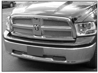
14. E&G recommends using a mild solvent to remove any glue residue from the grille surrounds. Use alcohol or glass cleaner to remove any solvent residue.
