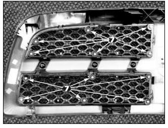
turn the grille over and tighten the #8-32 ESNA half nuts until the grille and mesh are snug. DO NOT OVERTIGHTEN or you could indent the mesh sur rounds at the stud locations.
