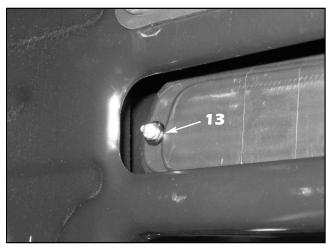
13. From underneath, install the small black plastic washers and the #8-32 ESNA half nuts and tight en. DO NOT OVERTIGHTEN or you will indent the grille at the stud locations.
