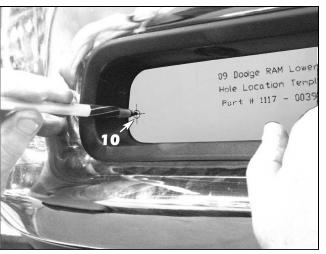
10. Align the lower template into palce and mark the outer hole location using an awl or similar pointed tool. Mark the hole on the opposite side by flipping the template over and aligning it into the opening.
