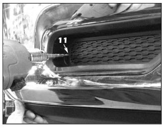
11. Use a 3/8" drill bit to drill through the marks made in the previous step.
