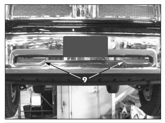
9. Align the mesh sections and the lower surround into the opening in the front bumper. Make sure the studs pass through the holes drilled in the previous step (mesh grille shown, "Q" similar).
