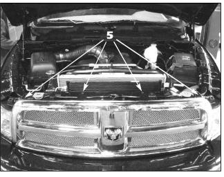
5. Reinstall the factory grille by clipping in the lower edge and reinstalling the four (4) 10mm hex head bolts.
