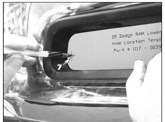
Align the lower template into palce and mark the outer hole location using an awl or similar pointed tool. Mark the hole on the opposite side by flipping the template over and aligning it into the opening.
