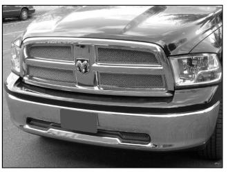
11.E&G recommends using a mild solvent to remove any glue residue from the grille surrounds. Use alcohol or glass cleaner to remove any solvent residue.
