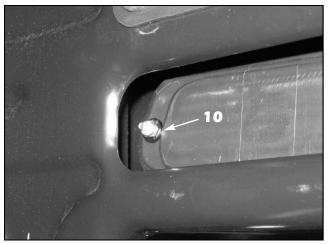
10. From underneath, install the small black plastic washers and the #8-32 ESNA half nuts and tighten. DO NOT OVERTIGHTEN or you will indent the grille at the stud locations.
