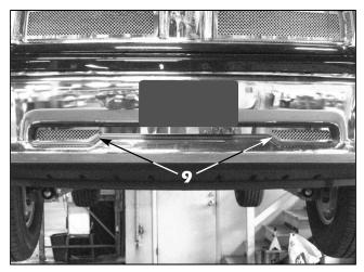
Align the mesh sections and the lower surround into the opening in the front bumper. Make sure the studs pass through the holes drilled in the previous step (mesh grille shown, "Q" similar).
