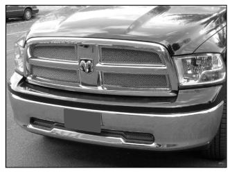
11.E&G recommends using a mild solvent to remove any glue residue from the grille surrounds. Use alcohol or glass cleaner to remove any solvent residue.
