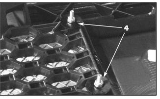
4. Install the stainless steel E&G grille sections into the openings on the factory grilles and tape them into place. Turn the grille over and install a large black plastic washer and a #8-32 ESNA half nut onto each mounting stud and tighten until snug. DO NOT OVERTIGHTEN or you will indent the grilles at the stud locations (mesh grille shown, "Q" grille same).
