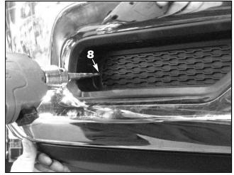
8. Use a 3/8" drill bit to drill through the marks made in the previous step.
