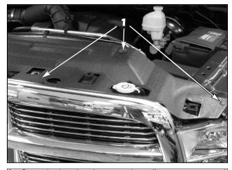
Open the hood and remove the radiator support panel cover exposing the factory hardware retaining the grille. Remove the plastic push pins by pulling straight up.
