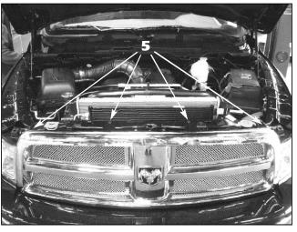
Reinstall the factory grille by clipping in the lower edge and reinstalling the four (4) 10mm hex head bolts.
