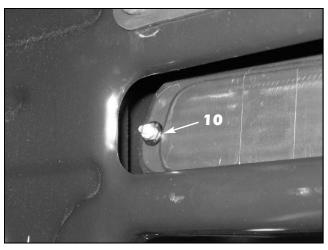
10.From underneath, install the small black plastic washers and the #8-32 ESNA half nuts and tighten. DO NOT OVERTIGHTEN or you will indent the grille at the stud locations.
