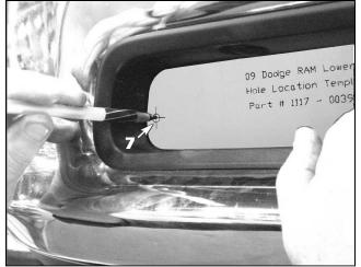
7. Align the lower template into palce and mark the outer hole location using an awl or similar pointed tool. Mark the hole on the opposite side by flipping the template over and aligning it into the opening.
