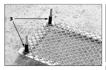
Remove the ends from the supplied black vinyl caps and slide them over the mounting studs on the grille sections (mesh grille shown, "Q" grille same). Align the mesh sections onto the backs of the stainless surrounds.
