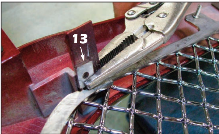
13. Align the upper mesh surround over the back of the mesh section and use vise grips to hold it in proper alignment. The surround should hold the mesh tight against the factory grille surround.
