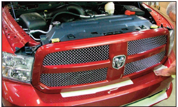
22. Finish the upper grille installation by clipping it back onto the grille support and reinstalling the upper 10mm factory fasteners removed in Step 3 . Replace the radiator support panel cover and remove the masking tape on the bumper cover. Upper grille installation is now finished.
