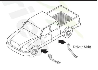
**4.** Install Front Mount Bracket by using one (1) Cab Mount Bolt.
