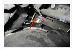
8. Using 13mm socket, remove the other 2 bolts securing the air box tray. Then remove the tray from the truck
