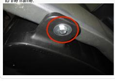
16. Reinstall the wheel liner using 5 of the OE screws and 3 supplied Panel Pins (Y). Reinstall wiring harness connector into wheel liner that was removed in Step #7.
