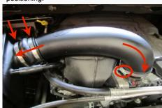
24. Reconnect the Temp. Sensor wiring harness.
