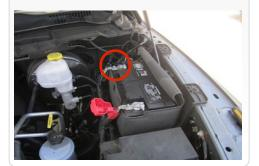
2. Disconnect the electrical connection for the Temp (IAT) Sensor. Note the sensor's orientation for the re-install.
