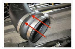
22. Secure the Silicone Step Coupler (B) to the throttle body using a #56 Hose Clamp (A). Place the #60 Hose Clamp (C) around the top of the Silicone coupler.
