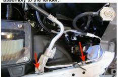
13. Carefully install the air box assembly into the truck at an angle as shown below.
