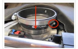
23. Insert the Intake tube assembly into the Silicone Coupler, then slide the Hump Adapter over the Adapter Tube. Tighten all hose clamps when you are satisfied with the positioning.
