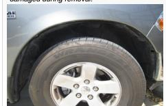
7. From inside the engine compartment, carefully pull the wiring harness connector out from the wheel liner. Then remove the wheel liner from the truck.
