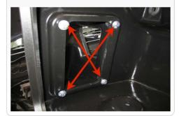
11. For those concerned about minimal engine heat; insert the Air Inlet Plug (T) into the end of the Air Inlet tube (S). Attach using the supplied 1/4"-20x3/4" screws (V), 1/4" Lock washers (U) and 1/4" Flat washers (W). For those seeking additional air flow, set the Air Inlet Plug aside and save all the supplied hardware. (See page 3 for more info and test results)
