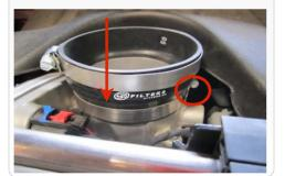
23. Insert the Intake tube assembly into the Silicone Coupler, then slide the Hump Adapter over the Adapter Tube. Tighten all hose clamps when you are satisfied with the
