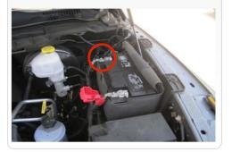
Disconnect the electrical connection for the Temp (IAT) Sensor. Note the sensor's orientation for the re-install.
