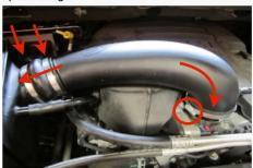
24. Reconnect the Temp. Sensor wiring harness.
