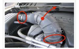
4. Remove the crank case vent tube from the air box.
