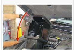
**14.** Using the OE bolt, secure the air box assembly to the frame. Leave loose for now..
