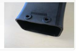
12. NOTE: Vehicles equipped with 4x4 can use the provided Screw Cap (O). Cut down and place on top of bolt accordingly to protect the S&B Air Box.
