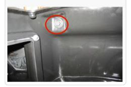
15. From inside the wheel well, attach the air box to frame using the supplied M8 x 40mm Hex bolt (K) and Fender Washer (L). Then secure both bolts mounting the air box
