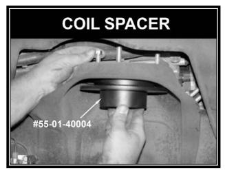
**NOTE:** On some models the driveshaft must be disconnected at the axle to allow the axle to drop sufficiently for coil / spacer installation.
