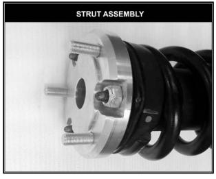
Raise the jack supporting the lower control arm. Loosely attach the lower end of the strut-tolower control arm using the factory hardware. Do not tighten at this time.
