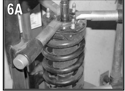
3/16" thick lockout tab onto the bolt; the tab seats in what was the factory rear cam washer's location. Install the supplied flat washer then the supplied 18mm Nyloc nut. Do not tighten. Note the crossmember goes inside of the factory mount.
