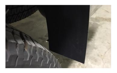
2. Align the flare on the fender lip for the amount of coverage and protection that is needed.
