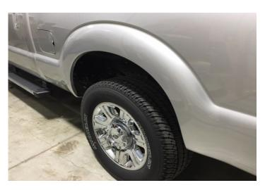
1. Clean the mounting location on your vehicle and check the location of factory fasteners and factory holes that can be used to fasten the flare. We recommend using the factory locations when possible then use the provided SS self tapping screws for further retention.
