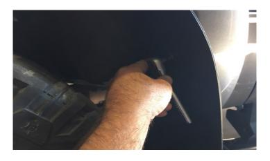
6. Fasten the flare to the truck with the factory fasteners. Check that the flare is parallel with the ground before tightening.
